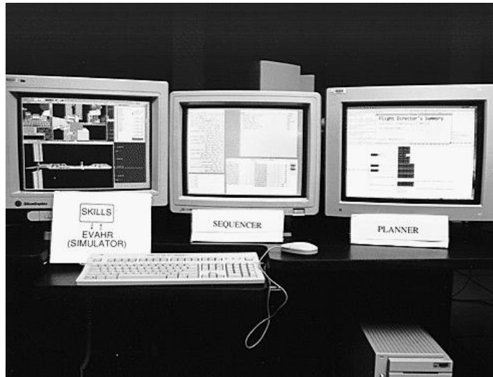
Figure 7.7 Each of the 3T layers running on a separate computer, controlling the EVAHR robot. (Photograph courtesy of the National Aeronautics and Space Administration, Johnson Space Center.)
