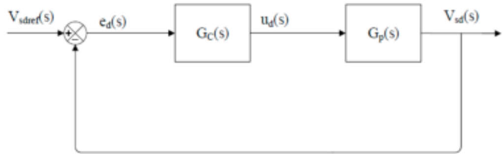
Figure 15. A block diagram for the VSC system AC voltage loop in a simplified form.
