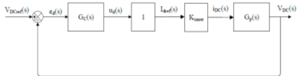
Figure 12. Simplified DC link voltage loop model of the VSC system.
