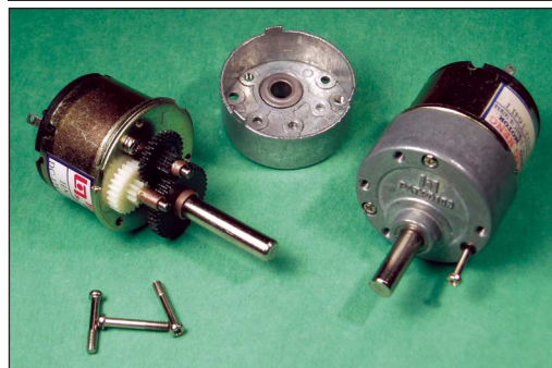
Figure 6. The 60-degree orientation mounting holes for the gearbox.
