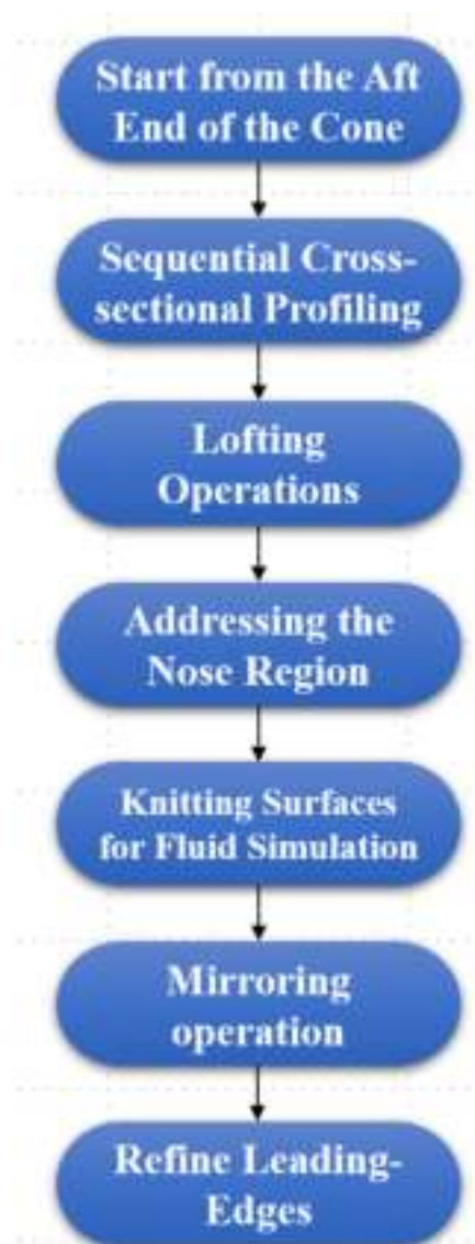
Figure 9. (Top): Waverider sections and the complete geometry. (Bottom): Flowchart of the design methodology.
