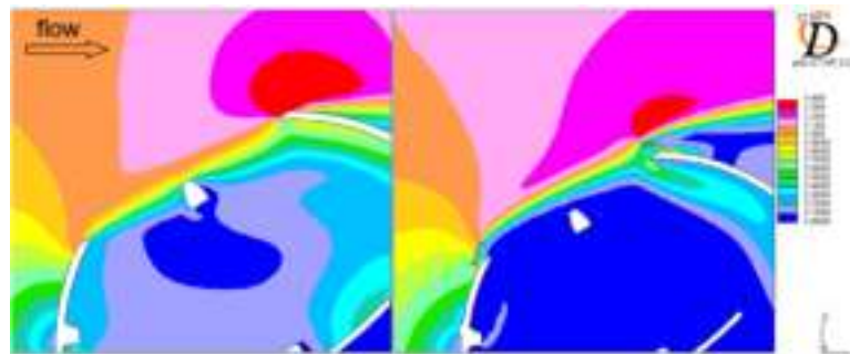
Figure 18. Impact of the TIO deflector design on velocity levels around the telescope top end (velocity scale normalized with upwind value).
