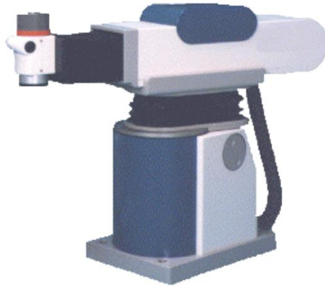
Figure 10 Le robot cylindrique RT3300 (Seiko)
