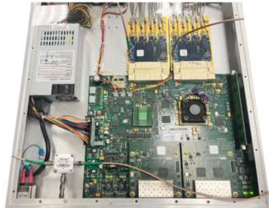
Figure 3. ROACH-2-based DSP platform based on Xilinx Virtex-6 Sx475 FPGA, and 32-channel ADC card. We gratefully acknowledge Dr. Dan Werthimer at UC Berkeley and the CASPER community for their contributions to the ROACH-2 and CASPER tools.
