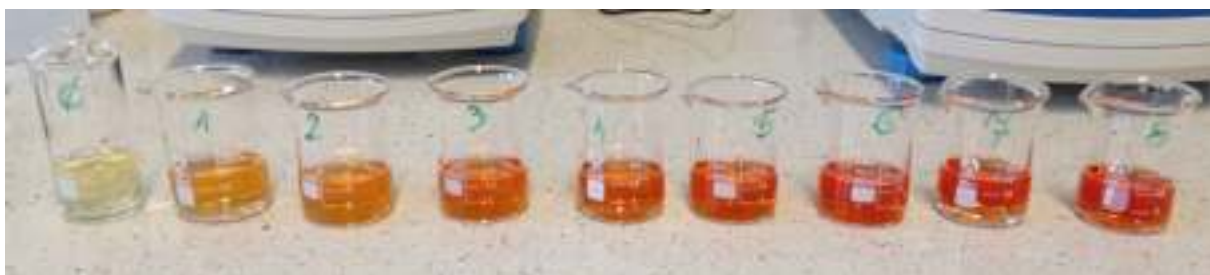
Figure 3. Vitamin C solutions (0, 4.54, 11.31, 18.05, 22.52, 33.63, 44.64, 66.37, and 87.72 \mu\text{g}\cdot\text{mL}^{-1} ) in the presence of double-distilled water, acetate buffer, ammonium iron(III) sulfate, and orthophenanthroline.
