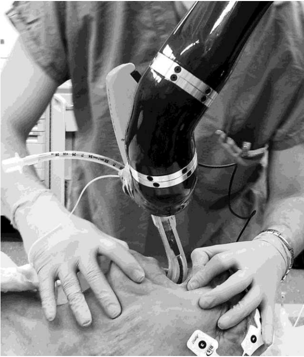
Figure 22.1 The Kepler intubating system (edited image from McGill University Medical Center. Accessed November 28, 2015 from https://muhc.ca/sites/default/files/news/DrHemmerling_KIS_closeup_20avril2011.jpg ). Courtesy of Montreal General Hospital MUHC.
