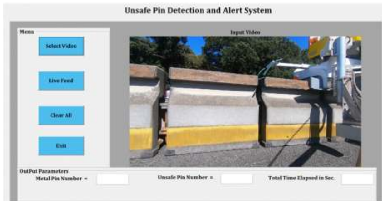
Figure 15. Graphical user interface for ‘Unsafe Pin Detection and Alert System’.
