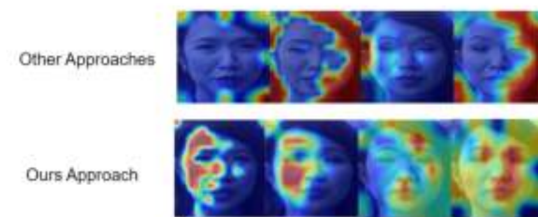
Figure 6. Comparison heatmap between other deepfake detector methods and our approach. From this figure, it is obvious that most deepfake detectors focus on boundary information of generated fake media.
