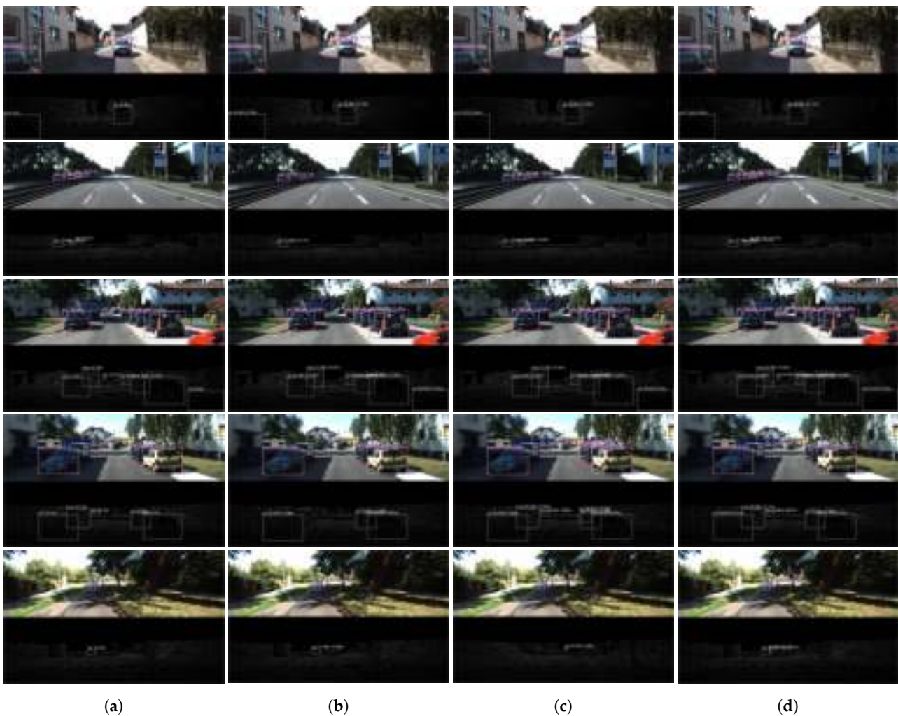
Figure 8. The visualization results of different monocular distance measurement methods. (a) is the ground truth. (b) is the result based on Faster R-CNN. (c) is the result based on YOLOv5. (d) is the result based on YOLO-RedeCa.
